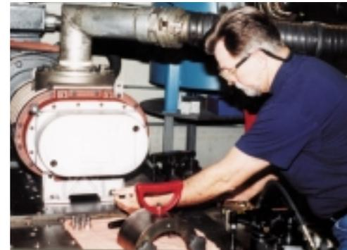
Prior to leaving the factory, every Legend is run tested against rigid standards using our advanced computer automated testing equipment.
