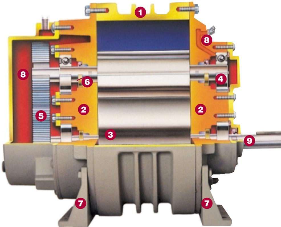
**1** High-strength impeller case is heavily ribbed and machined from a single piece of cast iron and features oversized dowel pins for precise mounting and alignment of head plates.
