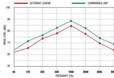
The sound data shown compares the Legend and a comparably sized blower operating at 3,275 rpm and 12 psig. An improved blower design significantly reduces the sound pressure output of the Legend blower. The typical reduction is 3 dBA which represents 50% less noise than the competition.
